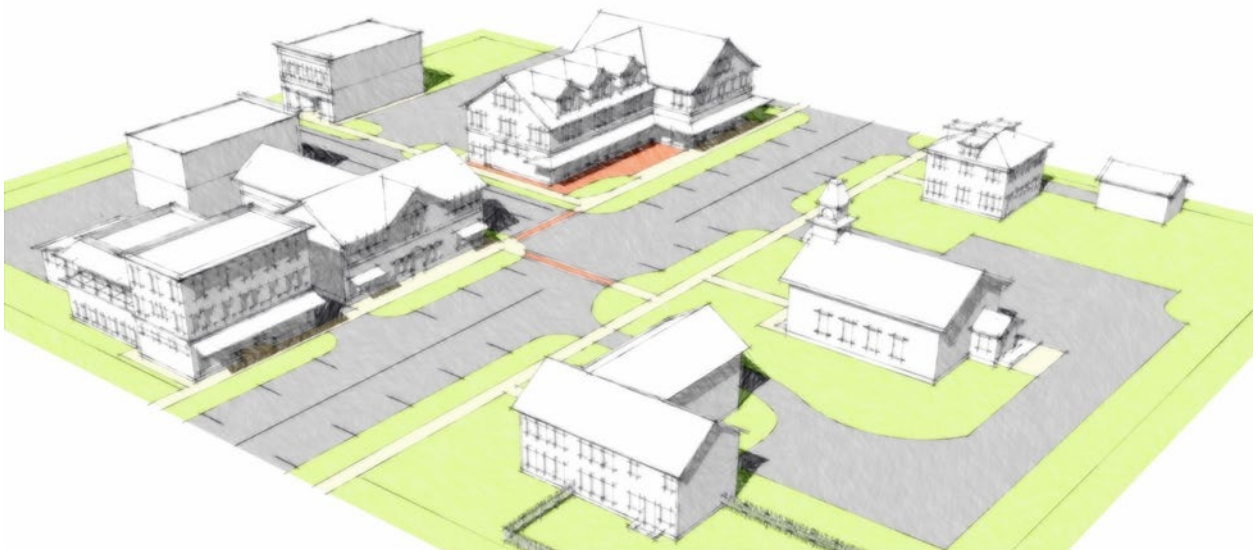
THIS: SHARED PARKING LOCATED TO THE REAR OR SIDE OF BUILDINGS WITH CROSS ACCESS BETWEEN LOTS
