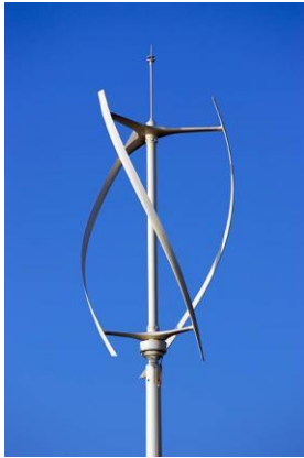
Figure 25: This photo is an example of a vertical axis wind
